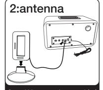
Snap AM antenna into provided stand, then plug antenna cable into socket on back of unit. Move antenna 12" away.
